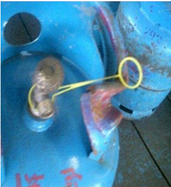
Fig.A.3.4 Example of collar damage
