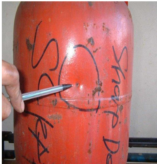
Fig.A.3.5 Example of gouge defect
