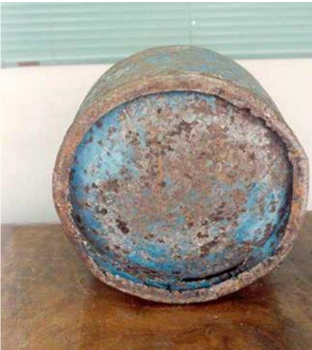
Fig. A.3.2 Examples of corrosion defects – General (right) and Corrosion pits (left)
