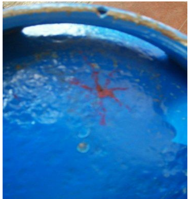
Fig. A.3.2 Examples of corrosion defects – General (right) and Corrosion pits (left)
