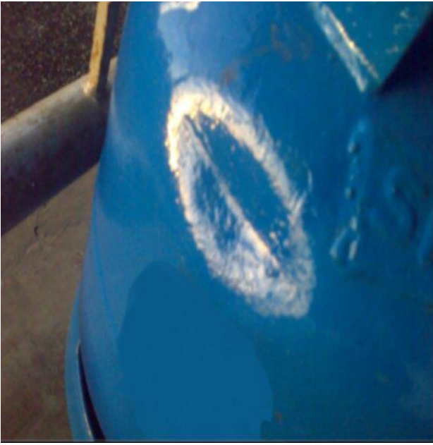
Fig. A.3.1 Examples of dent defects
